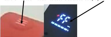
(FF displayed means the scooter is unlocked to a max speed 32km/h)
